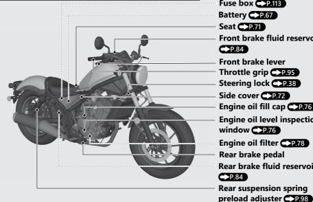
Fuse box P.113 Battery P.67 Seat P.71 Front brake fluid reservoir Front brake lever Throttle grip P.95 Steering lock P.38 Side cover →P.72 Engine oil fill cap P.76 **Engine oil level inspection** window P.76 Engine oil filter P.78 Rear brake pedal Rear brake fluid reservoir Rear suspension spring
