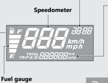
Remaining fuel when only 1st (E) segment starts flashing: approximately 0.58 US gal (2.2 L) If the fuel gauge indicator flashes in a repeat pattern or turns off: P.96
