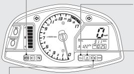
**Low oil pressure indicator**Comes on when the ignition switch is turned to the ON position. Goes off when the engine starts.
