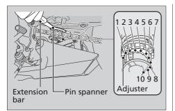
Attempting to adjust directly from 1 to 10 or 10 to 1 may damage the shock absorber.
