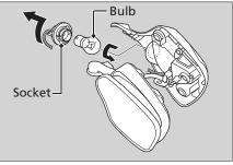
**6.** Install a new bulb in the reverse order of removal.
