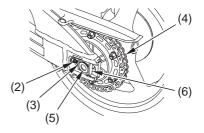
(4) drive chain(5) rear axle shaft(6) left chain adjustment plate
