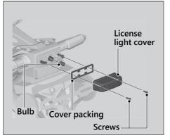
**3.** Install a new bulb and reinstall the parts in the reverse order of removal.
