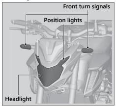
The headlight, position lights and front turn signals use several LEDs.
