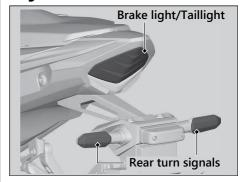
The brake light, taillight and rear turn signals use several LEDs.
