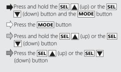
To set the ADJUST mode or LINE mode, press the **MODE** button. If the ignition switch is turned to the OFF position or none of the **MODE**, **SEL** (up) and **SEL** (down) buttons are pressed for about 30 seconds, the control is automatically switched from the setting mode to the ordinary display.
