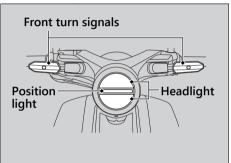
The headlight, front turn signals and position light use several LEDs.
