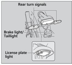
The brake light, taillight, rear turn signals and license plate light use several LEDs.
