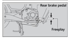
Make sure the brake rod, brake arm, spring and fastener are in good condition.
