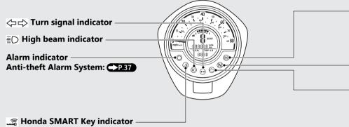
Comes on when vehicle and Honda SMART Key verification is complete, and the ignition switch can be operated. Goes off when the ignition switch is turned to the ON position.
