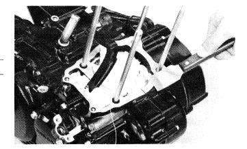
Install a new gasket and dowel pins.
