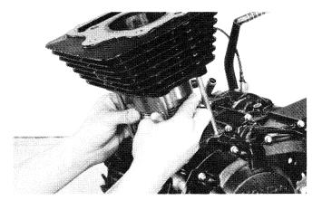
Tighten the cylinder mount bolts.
