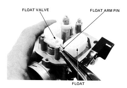
Inspect the float valve and seat for wear or damage. Replace them as a set if wear or damage can be seen.
