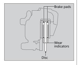
Inspect the brake pads from below the brake caliper.
