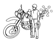
2. After warming up the engine, let the engine run at idling rpm for about one minute while the motorcycle is held upright.
