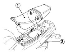
Lift the seat to make sure it is locked securely in position.
