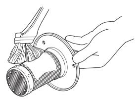
4. Install the spark arrester and gasket in the muffler, and tighten the bolts to the specified torque:
