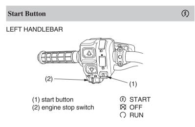
The start button (1) is used for starting the engine. Pushing the button in starts the engine. See *Starting Procedure*, page 69.
