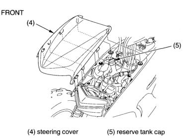
5. After adding coolant, install the reserve tank cap and steering cover.
