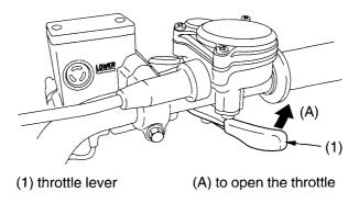
The throttle controls engine rpm (speed). To increase engine rpm, press the throttle lever (1) with your thumb. To reduce engine rpm, release pressure on the throttle lever. The throttle will automatically return to the closed position (engine idle) when you remove your thumb.
