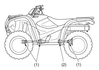
(1) rubber propeller shaft boots(2) rubber yoke joint boot
