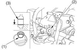
(1) oil drain plug(2) oil filler cap
