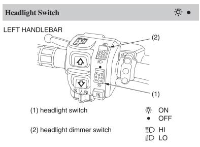
The headlight switch (1) is used to turn the headlight ON (  $\$ ) or OFF (  $\bullet$  ). To operate, turn the switch to ON (  $\$ ) or OFF (  $\bullet$  ).
