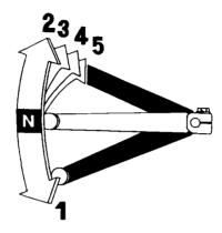
The gearshift pedal is located near the left footpeg. One full stroke of the pedal shifts the transmission to the next higher or lower gear in the shifting sequence. The pedal automatically returns to the horizontal position when released.
