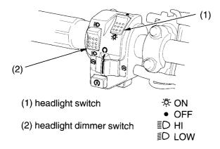
The headlight switch (1) is used to turn the headlight ON ( $^{*}$ ) or OFF ( $^{\bullet}$ ). To operate, turn the switch to ON ( $^{*}$ ) or OFF ( $^{\bullet}$ ).
