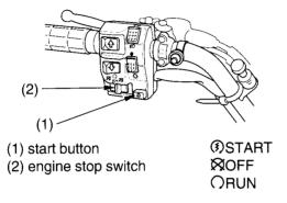
The start button (1) is used for starting the engine. Pushing the button in starts the engine. See *Starting Procedure*, page 61.
