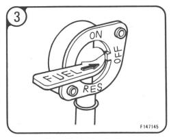
Turn the fuel valve lever to the "OFF" position.
