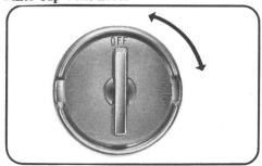
The fuel filler cap has a lever with "ON" and "OFF" positions to open or close tank vent.
