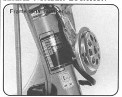
The frame serial number is stamped on the right side of the steering head. The engine serial number is stamped on the right side of the crankcase near the generator cover.
