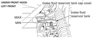
It should be between the MIN and MAX level marks. If the level is at or below the MIN level mark, check the brake pads for wear (page 130).
