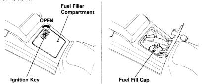
Use unleaded or low-lead petrol with a research octane number of 91 or higher. We recommend that you use unleaded petrol because it produces fewer engine and spark plug deposits and extends the life of exhaust system components.
