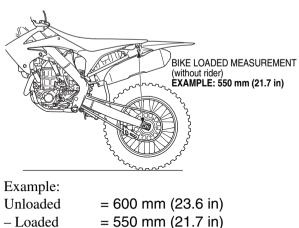
$\frac{-\text{Loaded}}{\text{Sag}} = 550 \text{ mm} (21.7)$   $\frac{-\text{Loaded}}{(21.7)} = 50 \text{ mm} (2.0 \text{ in})$  (Without Rider)
