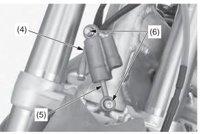
(4) steering damper(5) damper rod(6) steering damper mounting bolts
