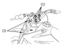
Operating the motorcycle with loose, worn, or damaged steering or front suspension components may adversely affect vehicle handling and stability.
