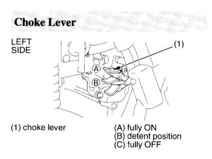
The choke lever is used for starting the engine (page 31). The choke increases the percentage of fuel in the fuel/air mixture delivered to the engine.
