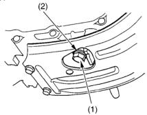
(1) oil drain bolt(2) sealing washer
