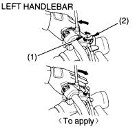
(1) rear brake lever (2) brake lock lever
