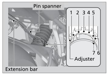
Attempting to adjust directly from 1 to 7 or 7 to 1 may damage the shock absorber.
