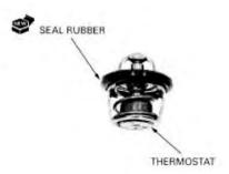
Install the thermostat into the housing with its hole facing up.
