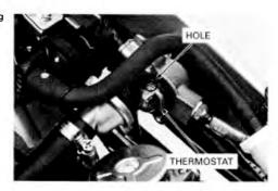
Install the thermostat housing cover and two bolts. Tightn the bolts securely.
