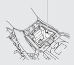
► The centre compartment may become heated by the engine. Do not store any items that are flammable or susceptible to heat damage.
