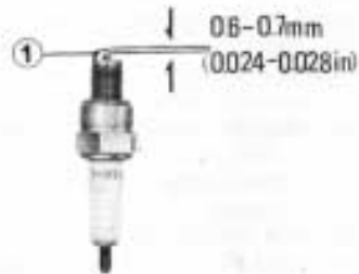
① Bend side electrode to adjust gap
